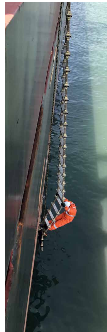
(left) Previous method of taking a Draft Survey was for a surveyor to scale down a rope ladder; (right) A surveyor using SGS's new DST Draft Survey Tool from the ship's deck
