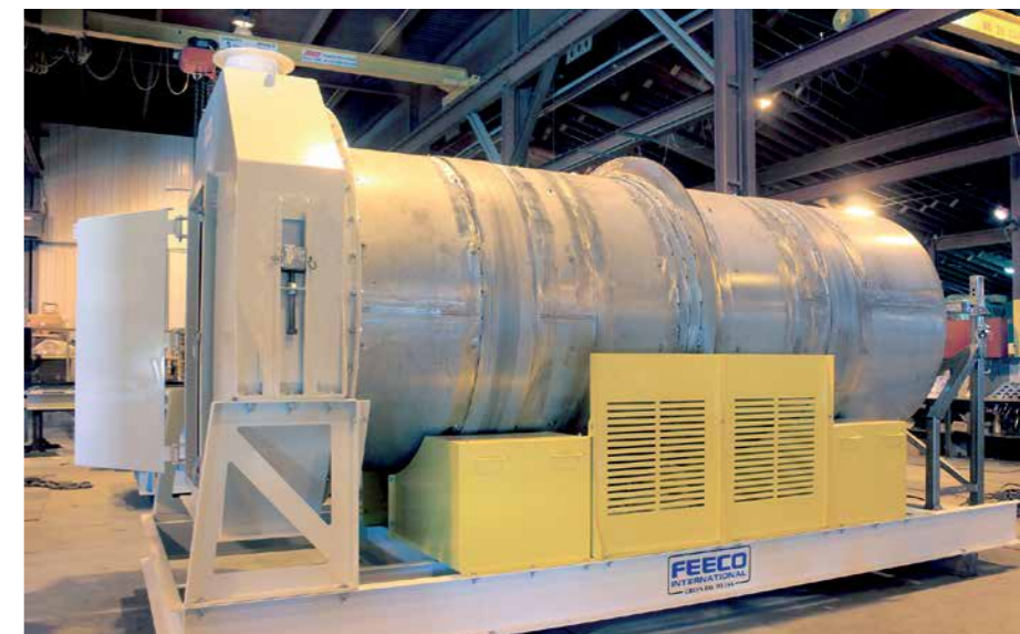
Coating drum in fabrication
