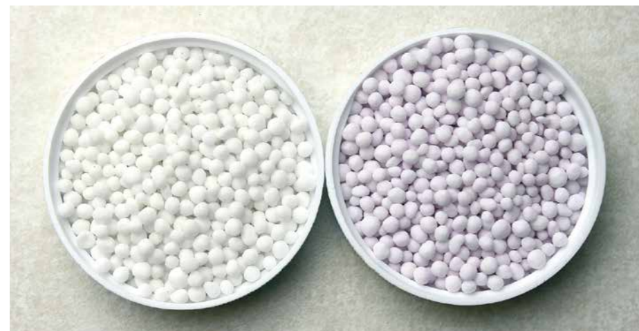
Urea before (left) and after (right) coating with an anti-caking agent
