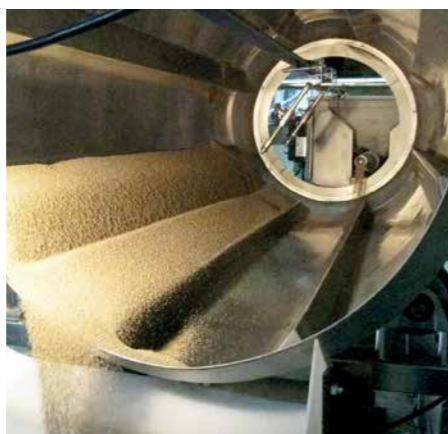
Interior view of a pilot-scale coating drum with tumbling flights used for testing in the FEECO Innovation Center
